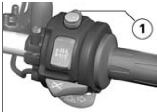
1 Emergency off switch (kill switch)
